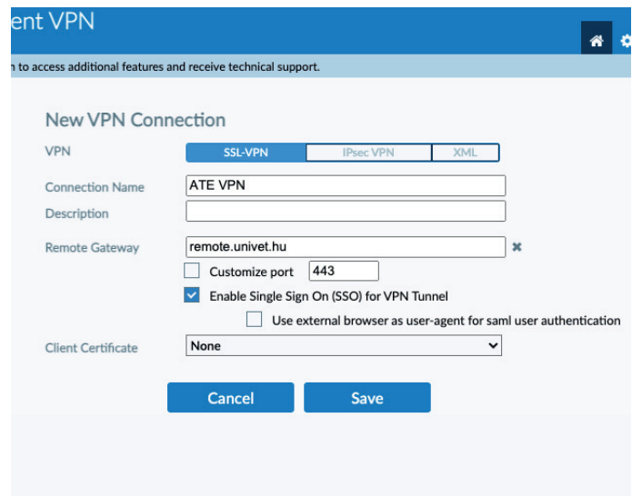
19. These are the configuration details what you need to fill in form.
